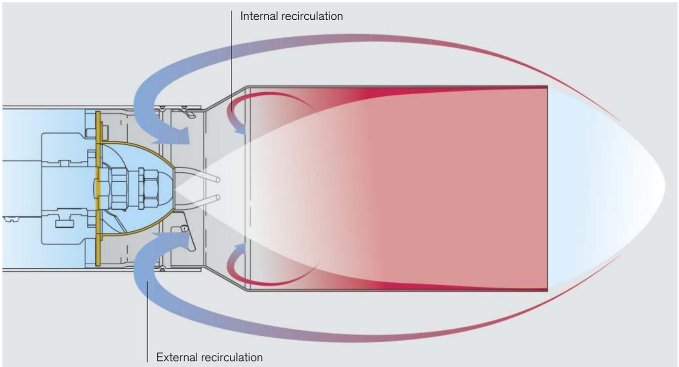
*The special construction of the mixing assembly effects the gasification of the oil mist and the necessary recirculation of the combustion gases – combustion of the oil is smoke free with considerably reduced NO<sub>x</sub> emissions*
